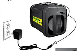
Turn on switch at top of unit. If LED indicates low battery, attach AC adapter & charge for 3-6 hours.
