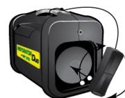
Retain lid for storage by placing against back of cartridge. Install spring-loaded latch bar into grooves, against cartridge lid, & twist to lock into place.
